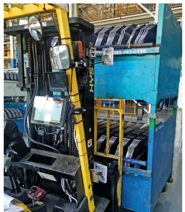
The UHF antenna on the truck identifies the container ID and updates the location in the WMS; the transport jobs are displayed directly on the monitor
